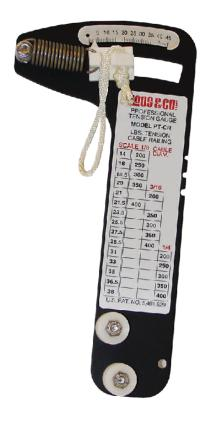
The Loos & Co. **Professional Model #PT-CR** tension gauge is designed to provide an accurate measurement of the tension in architectural cable railing systems.
