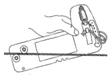
2. With the right hand pull the lanyard and extend the spring until the hook on the nylon slider can be hooked on to the cable as shown in **Figure 2**.
