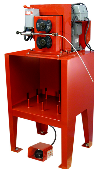
Figure II-4 Power driven machine with foot switch & electric cables mounted on top of shipping container/bench.
