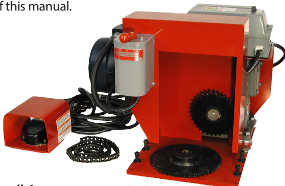
Figure II-6 Power Drive Kit laid out.
